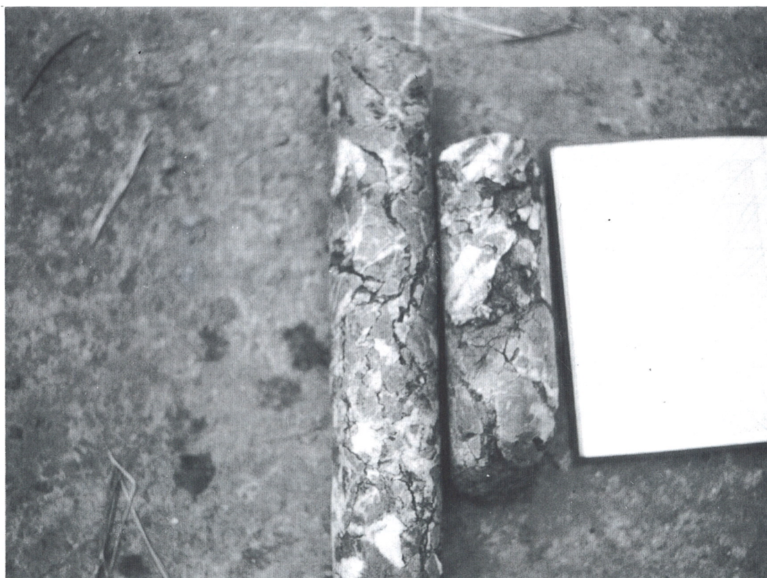
Photo 2 - Fault breccia at a depth of 9.9-11.0 m in borehole KH 104 affected by Fault F1 in the valley area
